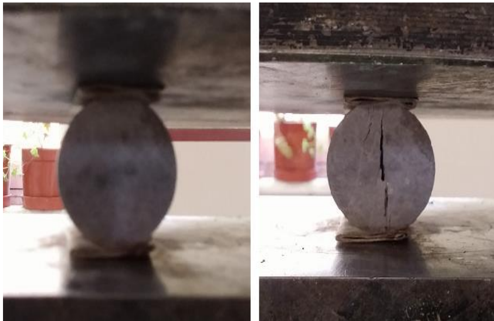
Fig 5. Indirect tension (Brazilian) tests
