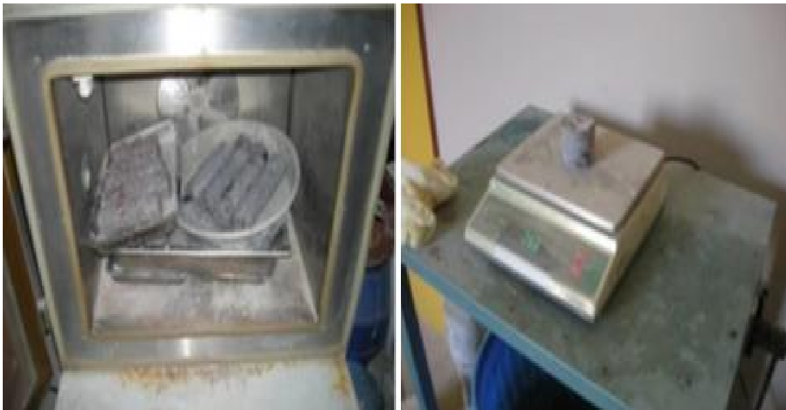
Fig 6. Drying in the oven and measuring the weight of samples
